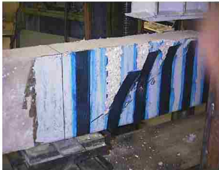
Figure 2.5. Shear Failure due to FRP Debonding (Khalifa, 1999)
